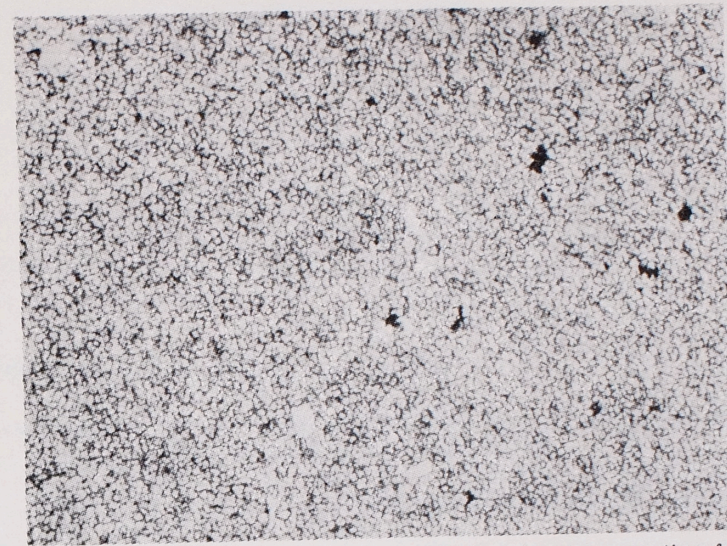
Phot. 1. Homogeneous, fine-crystalline structure of carbonate concretion from Hieroglyphic Beds. 1 nicol. Magn. \times 80
